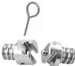
the tool attachment key supplied with the machine should be inserted into the side boring of the coupling on the spirals
